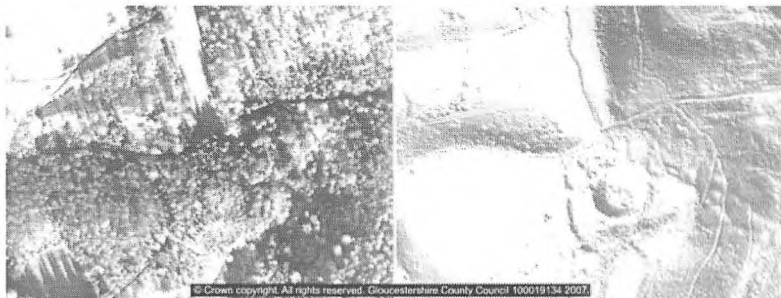
A typical aerial photograph and a LIDAR surveyed ground surface of the same area.
