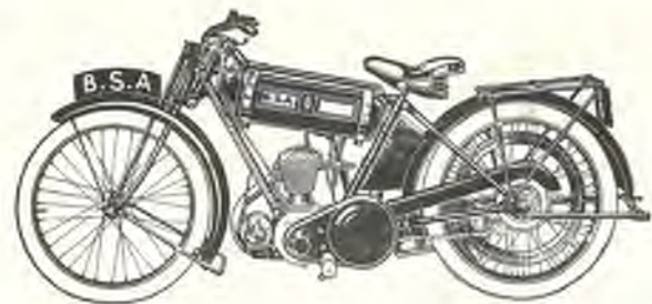
2.49 h.p., 4-stroke, 2-speed, clutch, k.s., mechanical oil pump, all-chain drive. 35 gns.
