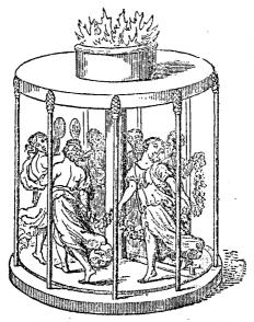
What the steam engine was two thousand years ago may readily be gathered from the above engraving; in short it can only be characterised as a pleasing philosophical toy, put in operation by steam or compressed air. The figures were made to revolve on the principle of the common rocket wheel, the fire being applied above as shown in the sketch.
