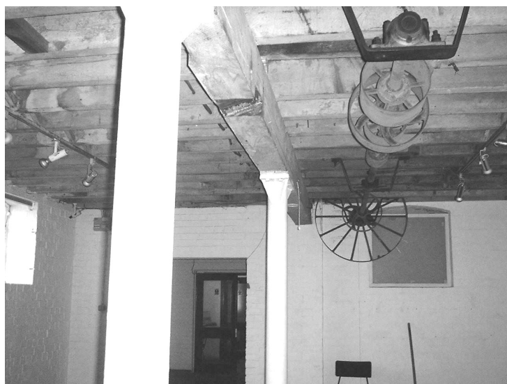
Original line shafting inside the Axiom [photograph courtesy of Klara Sudbury]
